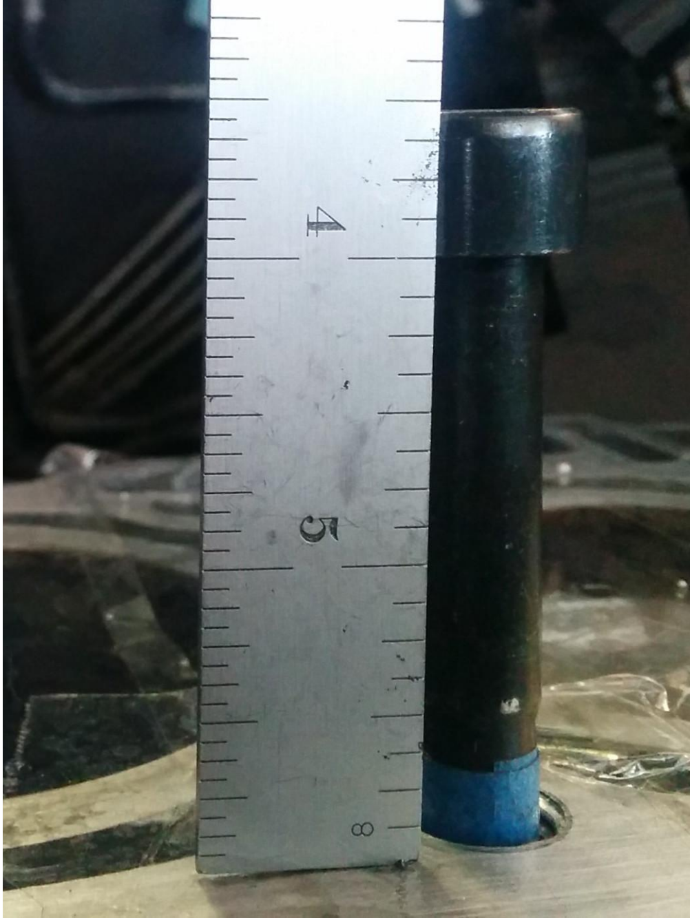
Figure 23: Check the head bolt will screw in far enough
