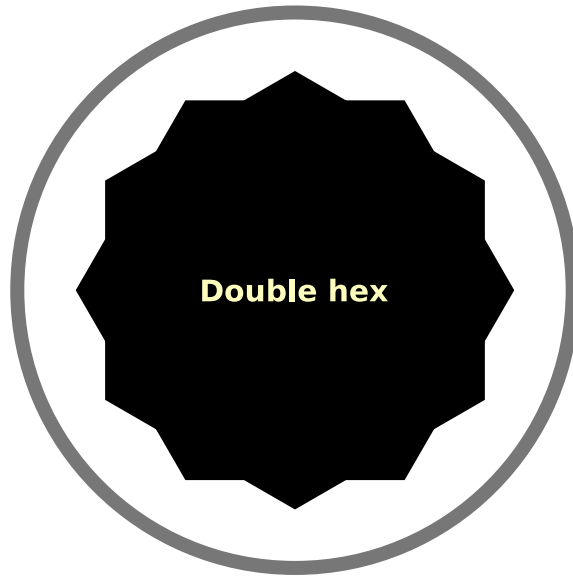
Figure 9: The shape of a double-hex driver
