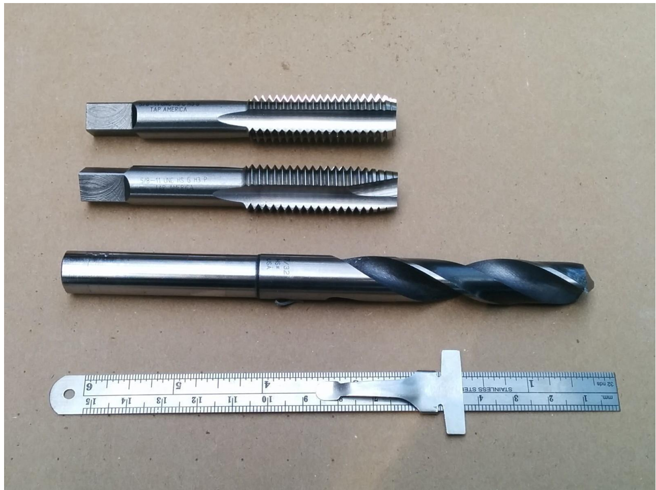
Figure 3: A 17/32" drill, and two 5/8" x 11 taps (one plug, one bottoming)
