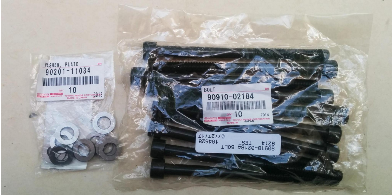
Figure 13: Toyota head bolts
