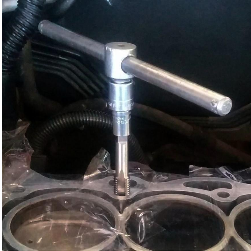
Figure 19: Remove the jig block and tap the rest of the way
