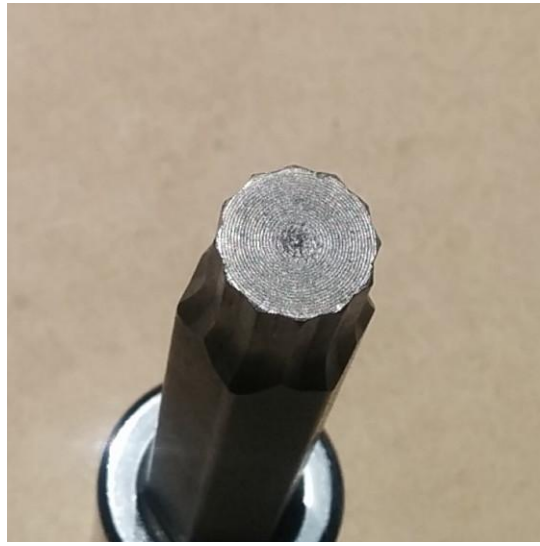
Figure 7: The correct double-hexagon socket driver
