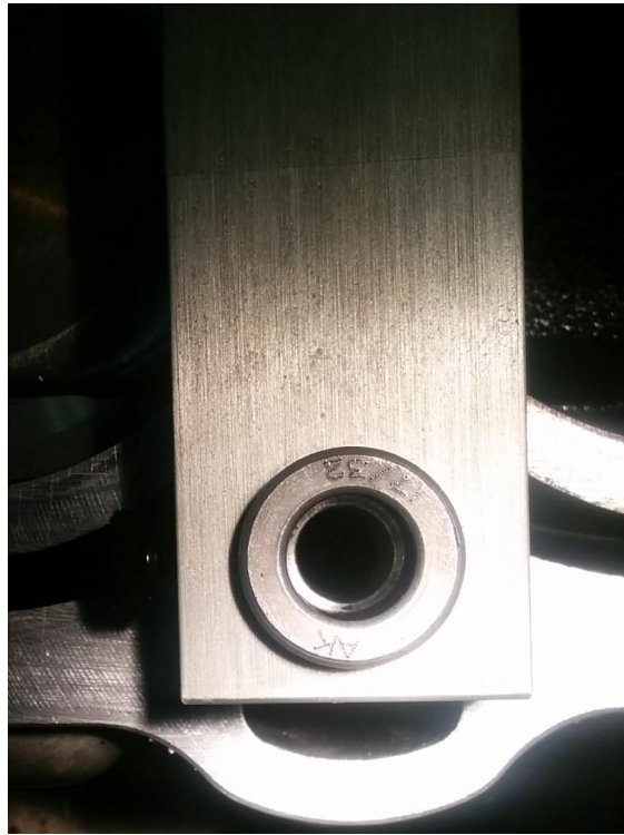
Figure 15: Jig block visual check before drilling
