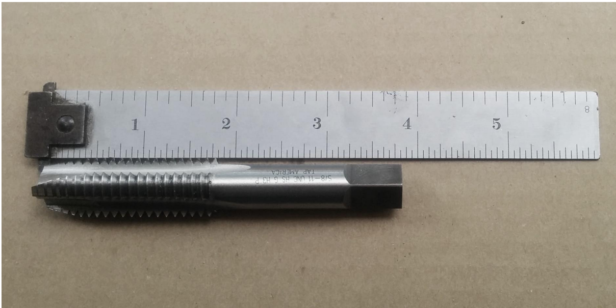
Figure 20: The tap is 3 13/16" long
